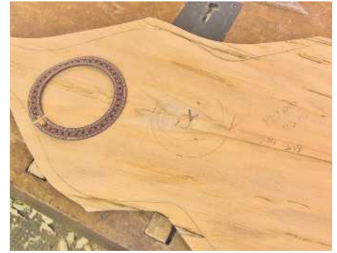
▲ Pic.3 Mark out the sound hole – careful measurement is needed to find the centre location!
